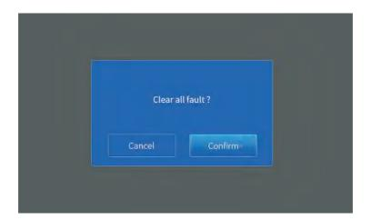
Press the "Confirm" key, you can delete the fault record.
