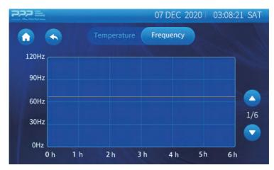
The curve is saved every 5 minutes, and the curve record can save data for 60 days.
