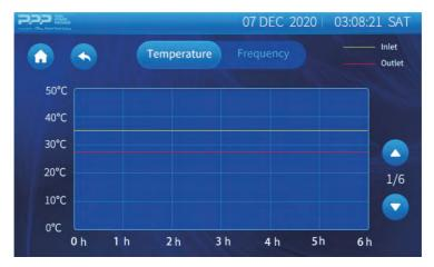
Click "Temperature" to check the state of the Temperature curve; Click "Frequency" to view the compressor's Frequency curve.
